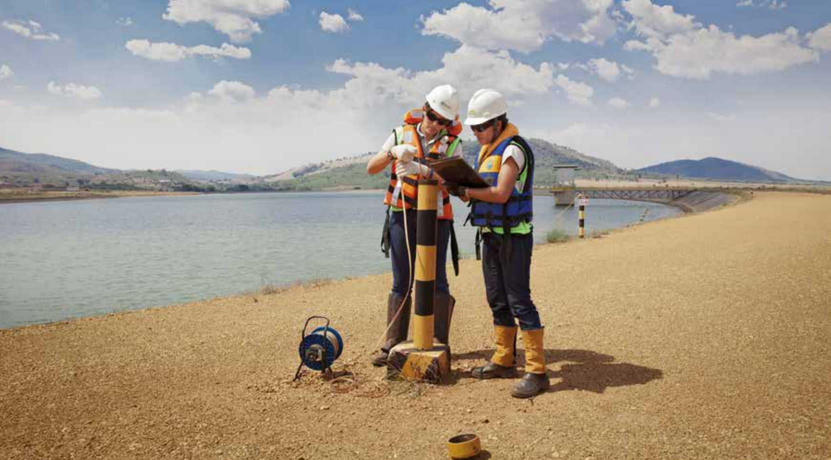
Hamanda Jansen (left) and Anita Marques, environmental engineers, measure the water height at Barro Alto dam in Brazil.
