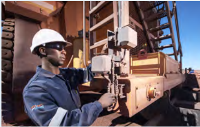
Fitment technician, George Phirimi, inspects the radar sensors, which are fitted front and rear, and cameras for the auto-braking system on a Komatsu 730 haul truck.
